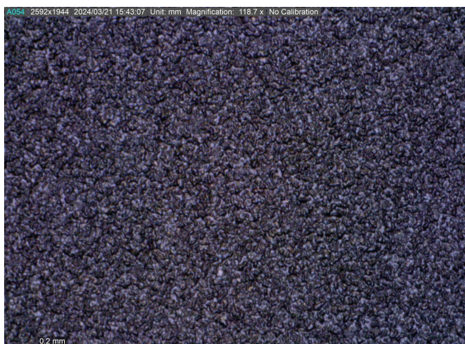
FIGURE 1 Polyester/GMA acrylic close-up showing microtexture of the surface
