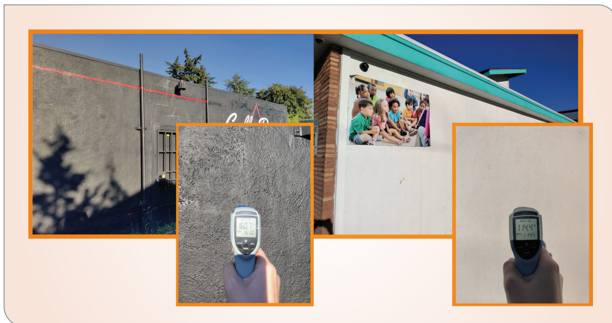
FIGURE 3 Difference between the surface temperature of a dark exterior wall (160.7 °F) and a light exterior wall (114.4 °F) on July 19, 2022, at 7 p.m. in Portland, OR.
