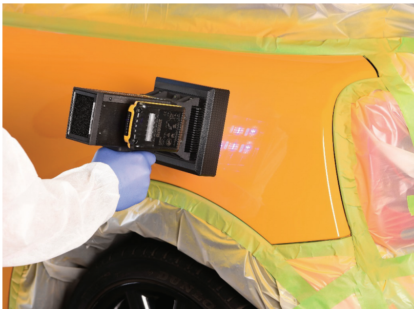
FIGURE 16—Integration Technology AC-500 battery-powered portable UV LED handset for small-damage repair.
