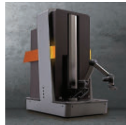
The PictoBot robotic painting device. Source: Transformarobotics.com
