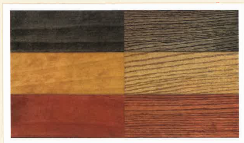
Figure 4 —Transparent iron oxides are chemically identical to their opaque counterparts; it is the crystallization process that creates the transparent effect. Extremely durable, lightfast pigments, the UV-curable Lucida Colors™ Trans-Oxide™ pigment dispersions shown here in black, yellow, and red (10% dispersion on left, 5% on right) have a 7-8 wood scale rating and showcase the wood grain.
