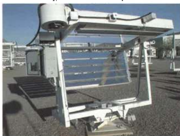
FIGURE 7—Fresnel-type accelerated outdoor exposure device.
