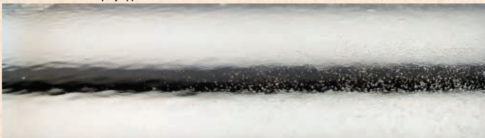
FIGURE 1—Pinholes in a Spray Applied Automotive OEM Basecoat
