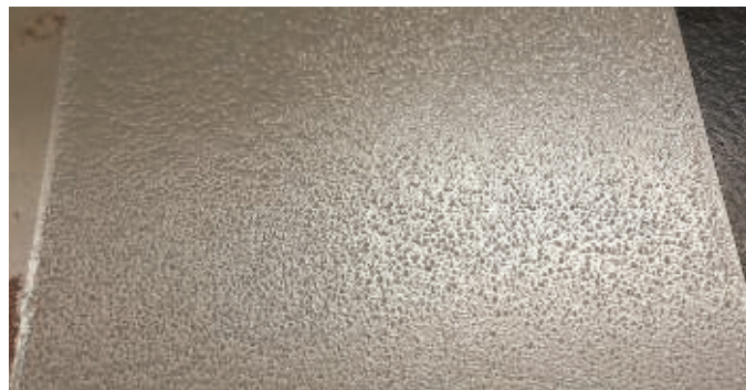
FIGURE 1—Low-VOC 2K polyurethane clearcoat over cold rolled steel substrate, exhibiting low gloss and microfoam.
