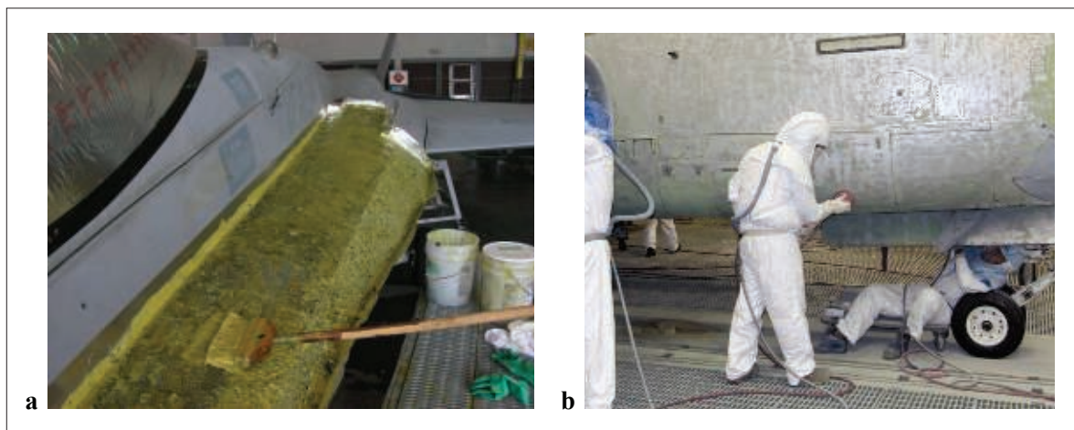
FIGURE 1 —Removal of the crosslinked polyurethane coating on Navy aircraft using (a) a methylene chloride-based paint stripper and (b) mechanical sanders.
