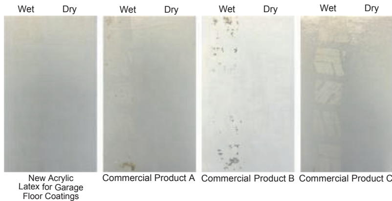
FIGURE 2—72-hour cure hot-tire resistance test blocks.
