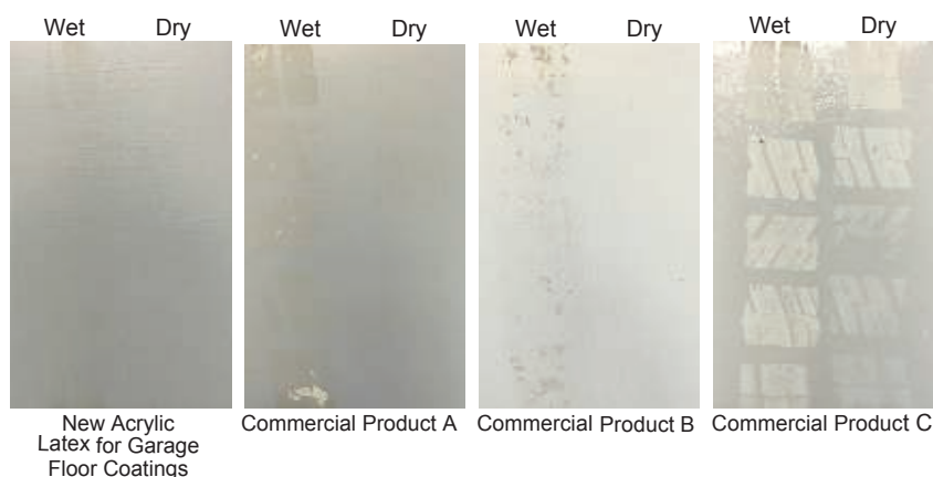
FIGURE 1—24-hour cure hot-tire resistance test blocks.
