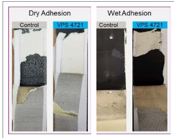
FIGURE 6 —Failure mode analysis of the waterborne acrylic roof coatings during dry and wet adhesion testing on aged EPDM. Adhesion failure was observed on both control samples, while cohesion or mixed failure was observed when the epoxy-functional silane oligomer was present in the coating.
