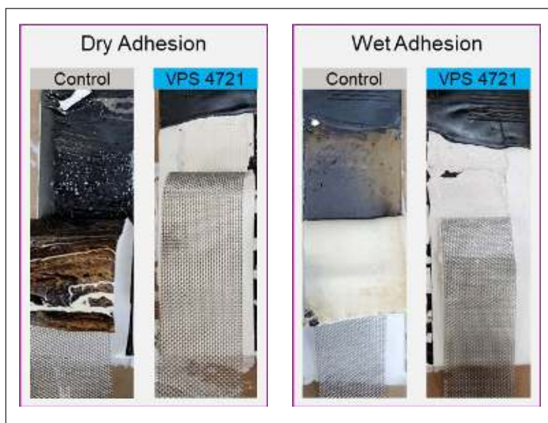
FIGURE 8 —Failure mode analysis of the waterborne acrylic roof coatings during dry and wet adhesion testing on aged asphalt. Adhesion failure was observed on both control samples, while cohesion failure was observed when the epoxy-functional silane oligomer was present in the coating.
