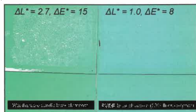
Figure 2—Phthalo green tint latex formulations with clearcoat of the same resin after QUV-B (313 nm) exposure (7000 hr for PVDF-based coatings, 5500 hr for acrylic coatings). Bottom portion is unexposed paint color. No UV absorbers were added to these formulations.
