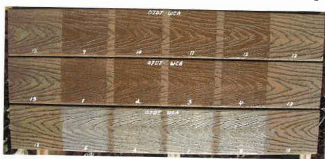
Figure 10—WPC-1 panels after eight months' exterior exposure. Top—Resin A; Center—Resin C; Bottom—Resin B. L to R: no coating→coating, no LS→LS Blend→UVA-1/HALS-1→UVA-2/HALS-1→no coating.
