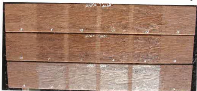
Figure 12—WPC-2 panels after eight months' exterior exposure. Top—Resin A; Center—Resin C; Bottom—Resin B. L to R: no coating→coating, no LS→LS Blend→UVA-1/HALS-1→UVA-2/HALS-1→no coating.
