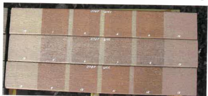
Figure 11—WPC-2 panels after three months' exterior exposure. Top—Resin C; Center—Resin B; Bottom—Resin A. L to R: no coating→coating, no LS→LS Blend→UVA-1/HALS-1→UVA-2/HALS-1→no coating.
