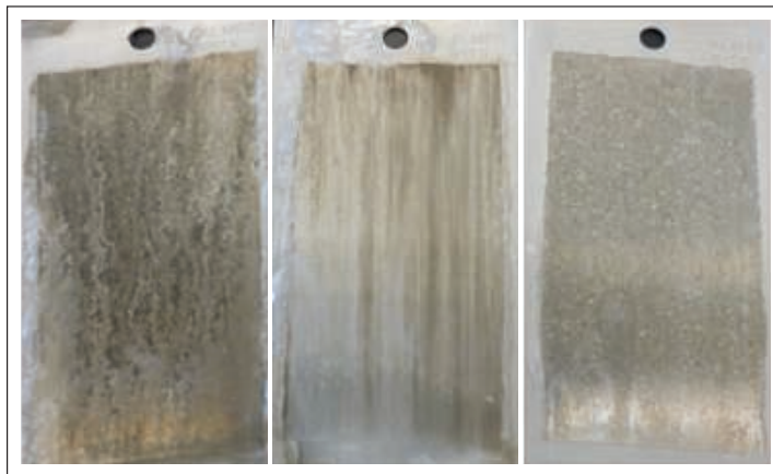
FIGURE 7 —WB2-coated aluminum after 250 h in a neutral salt spray test. Coatings cured for 72 h at 23°C (left), 30 min at 80°C (middle), and 30 min at 180°C (right).
