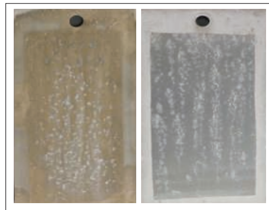
FIGURE 14—WB2-coated aluminum (left) and WB3-coated aluminum (right) after an alkaline resistance test and 100 h in neutral salt spray testing.
