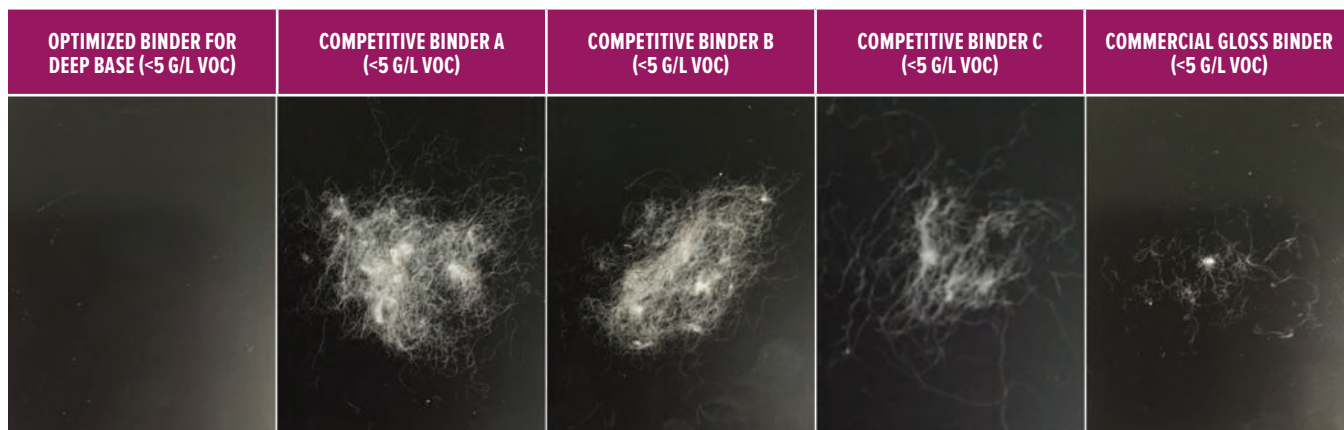
FIGURE 3 —Photographs of coated test panels after removal of cotton balls that were placed on each panel and subject to 15 min of pressure from a 1000 g weight.
