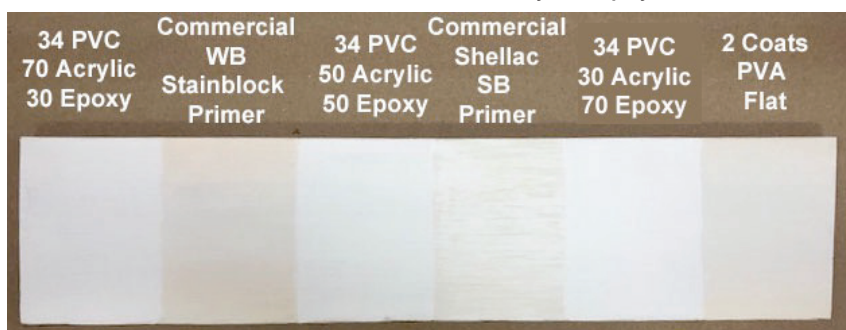
FIGURE 5—Tannin stain resistance on redwood: blend ratios of acrylic and epoxy, 34% PVC.
