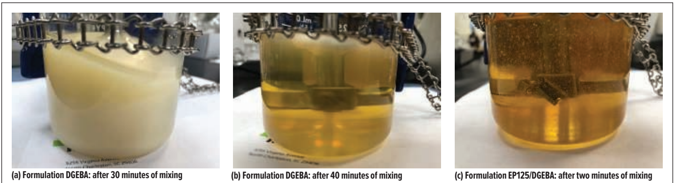
FIGURE 2—Mixing Comparison Between DGEBA and Versamid 140 With and Without DTO-based Epoxy
