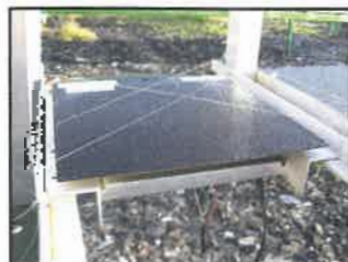
Figure 4—Panel with dew formation.
