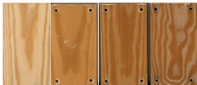
Figure 2—Progression of checking and discoloration within southern pine samples exposed to 0, 486.8, 939.4, and 1363 MJ/m 2 of irradiation (left to right), respectively.
