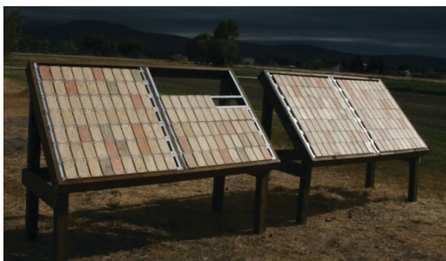
Figure 1—Samples mounted on 45° racks and pointed due south in Klamath Falls, Oregon, prior to the installation of the sprinkler heads.
