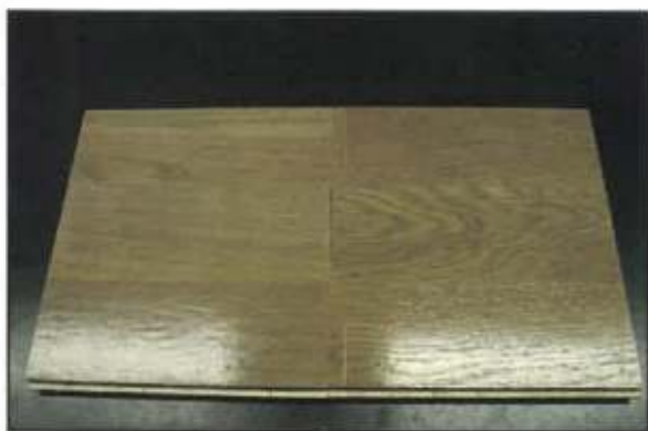
Figure 14—1-K water-based lacquer formulated on resin No. 2 without (left) and with (right) 20% SiO 2 addition of epoxy-silane modified colloidal silica.
