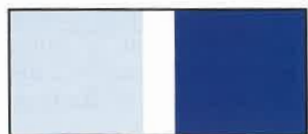
Figure 3—Unexposed FWT-60 film, OD .03 (left), and exposed film, OD 1.65 (right).
