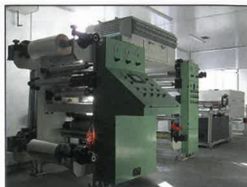
Figure 6—Sequential processing instrument for superhydrophilic films with UV lamps.
