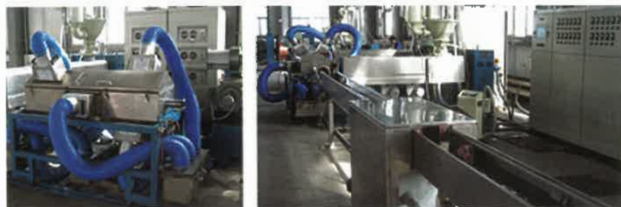
Figure 5—UV irradiation unit and production line of cable.
