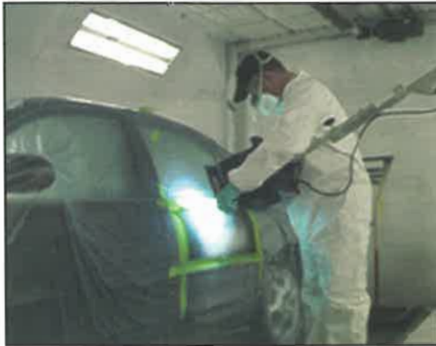
Figure 2—H&S AutoShot 400 UVA lamp used in body shop and lab.
