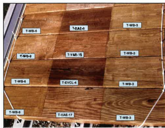
Figure 7—ACQ pressure treated decking boards after 12-month exposure at horizontal in Allentown, PA.
