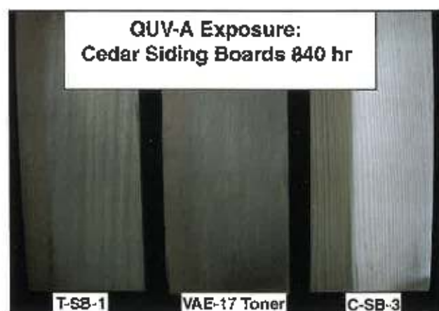
Figure 2—Cedar plank specimens after five weeks exposure in QUV-A.
