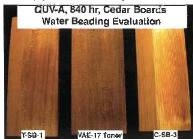
Figure 3—Cedar plank specimens after five weeks exposure in QUV-A with water spray to evaluate water beading.
