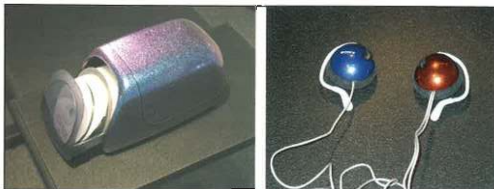
Figure 9—Coatings containing DOVP over black background.
