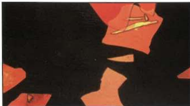
Figure 6—An optically variable pigment based on 80 micron-sized borosilicate substrate with high-low-high dielectric stack structure surrounding the substrate.
