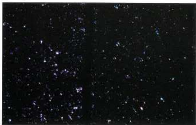
Figure 7—A DOVP (left) vs. a blend of red, blue, and gold borosilicate-based interference pigments (right).
