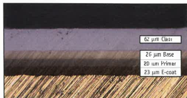
Figure 11—Cross section of a four-layer automotive coating on steel.
