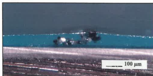
Figure 10—Cross section of an automotive coating showing overspray particles in the clearcoat.
