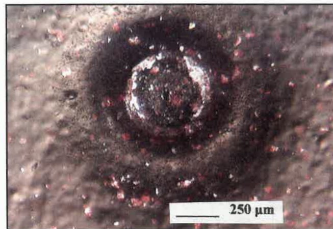
Figure 6—Gassing from a plastic substrate.
