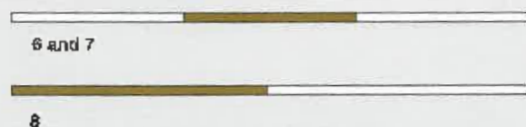
Scheme 4—Polybutyl acrylate polysiloxane block copolymer structures 6–8. □ = polyacrylate and ■ = polysiloxane.
