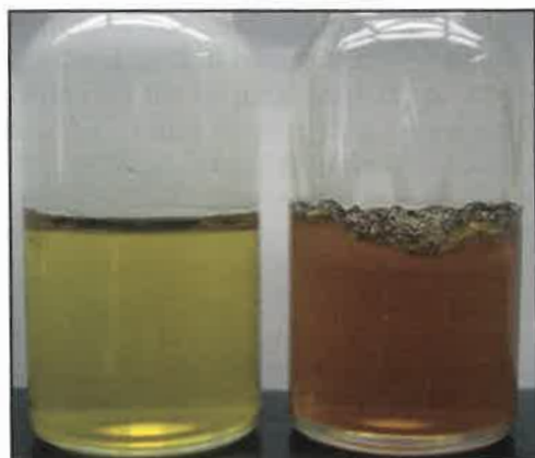
Figure 4—Tung oil only (no cobalt; left image) and skin formation in tung oil using MEKO after four days (right).
