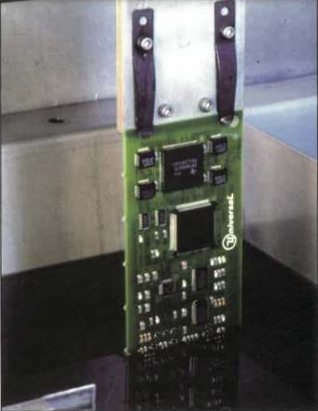
PC boards can be dipped into silicone-based conformal coating materials to protect the boards and their chips. Typically used for medium- to high-volume production, dip coating can assure complete coverage of a circuit board. (Photo courtesy of Dow Corning Corp.)
