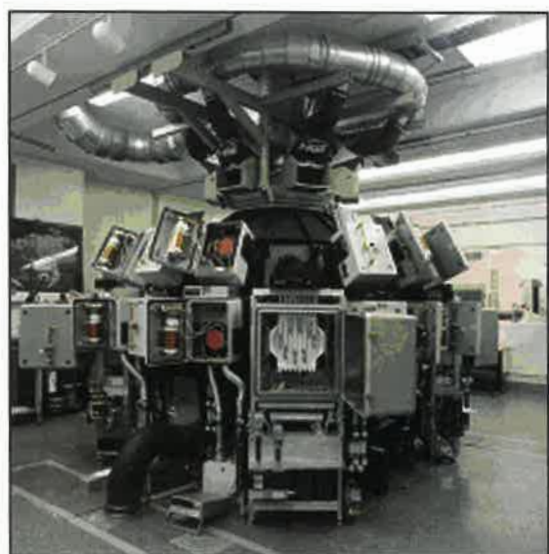
Figure 1—NIST 2 m integrating sphere, shown with UV light source and environmental chambers.
