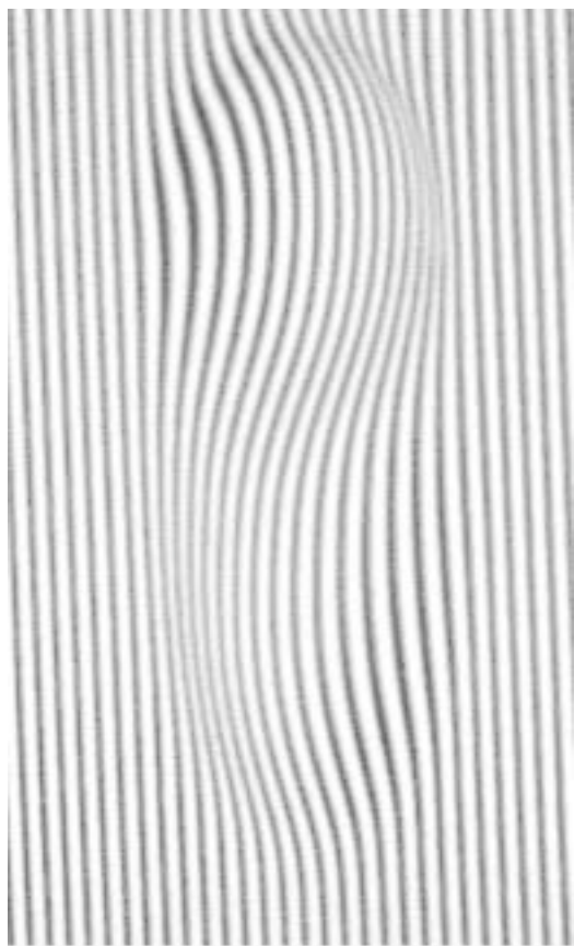
Figure 4—Image of dripmark with projected Ronchi ruling array.
