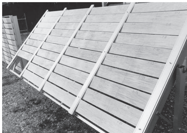
Figure 1—White test paints and controls applied one coat without primer on southern yellow pine, exposed on aluminum racks at 45° south in Huber, GA.
