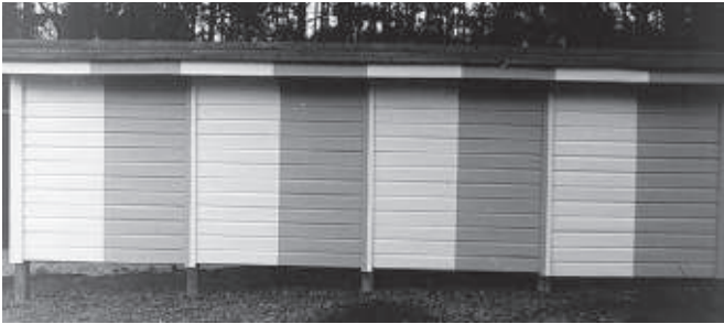
Figure 3—White and gray test paints and controls applied two coats over latex primer on southern yellow pine, exposed on test wall at south vertical in Huber, GA.
