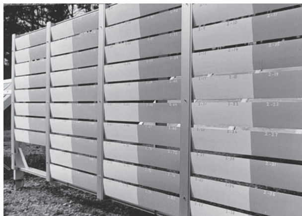
Figure 2—White and gray test panels and controls applied two coats over latex primer on southern yellow pine, exposed south vertical in Huber, GA.
