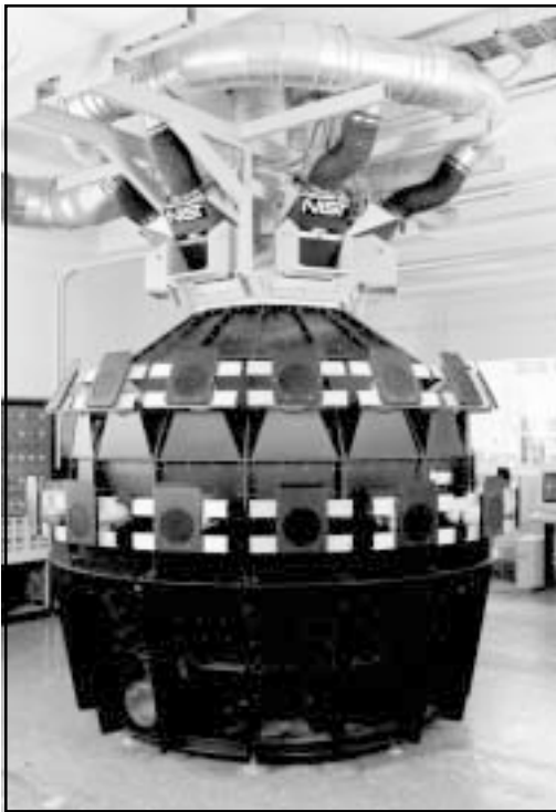
Figure 2—NIST 2 m integrating sphere, shown with UV light source.
