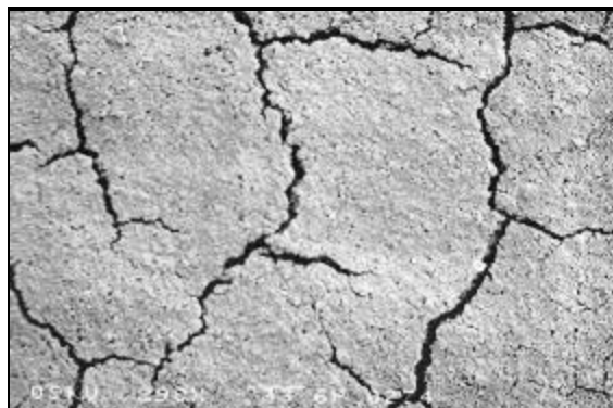
Figure 6—SEM of surface of silica-PVOH (203) coating.
