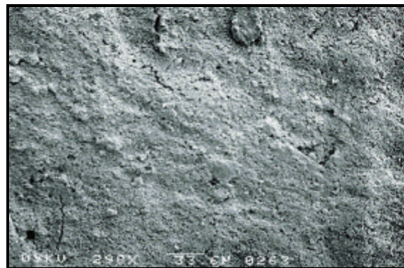
Figure 8—SEM of surface of SEAS-PVOH (203) coating.
