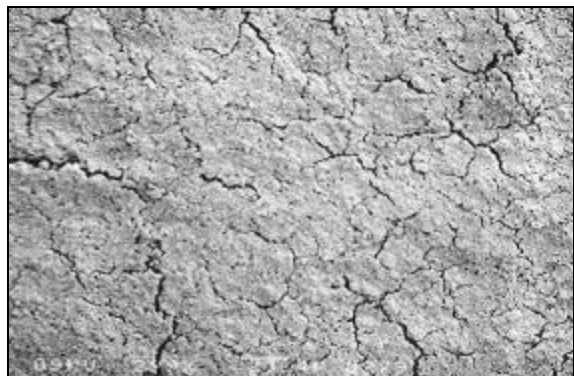
Figure 5—SEM of surface of silica-PVOH (103) coating.
