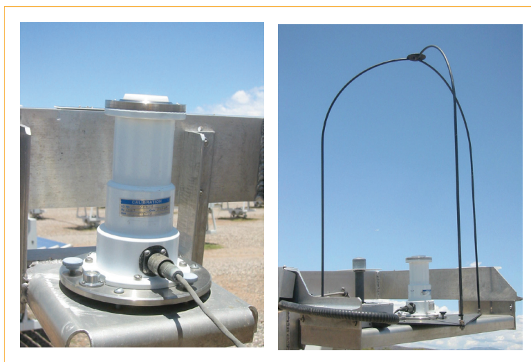
Figure 8 —UV radiometers in unshaded and shaded configuration.
