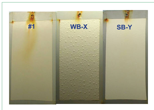
Figure 4—CRS panels after 1,008 hr of immersion in DI water.
