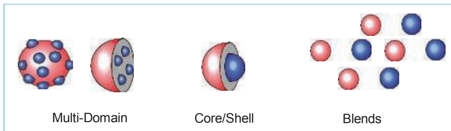
Figure 2 —Different latex morphologies are possible technical approaches to balancing VOC levels and hardness properties.
