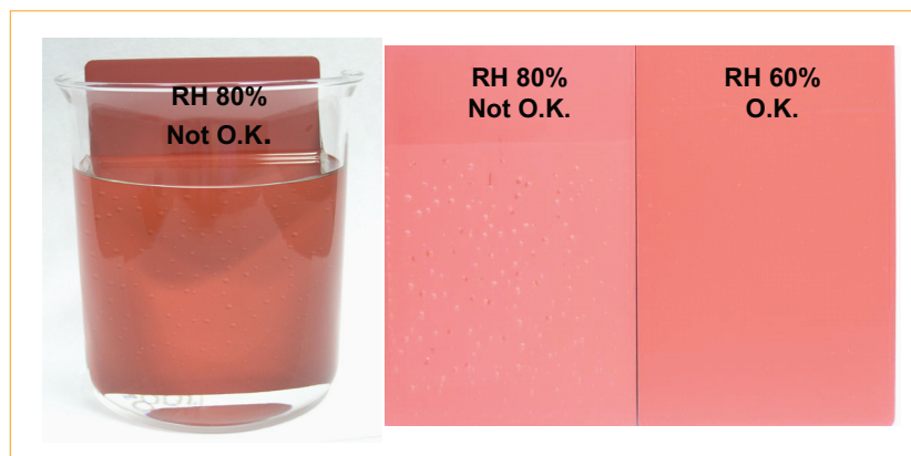
Figure 3 —Effect of RH on the early water-spot resistance of commercial anticorrosive paints. Application of the waterbased coating under high RH conditions can lead to strong blistering and early failure of the coating.
