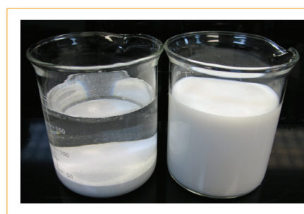
Figure 2 —Aluminum oxide dispersions in TPGDA with different surface treatments resulting in either poor dispersion and flocculation of the particles (left), or a stable and compatible dispersion of nano-particles (right).
