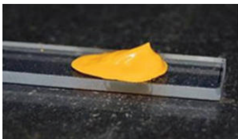
Figure 3 —Paste of cadmium sulfide/selenide-coated \text{TiO}_2 quantum dots.
