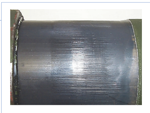
Figure 6 —Damaged Nylon 11 coating after 25,000 actuations in sand.
