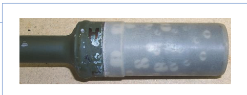
Figure 10 —ATP coating after impact and testing.
