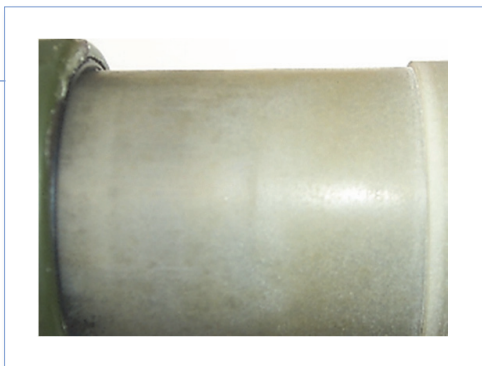
Figure 7 —Undamaged ATP coating after 25,000 actuations in sand.
