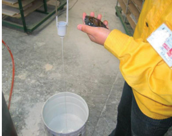
Figure 3 —Paint viscosity is measured by timing how long it takes for a known volume to drain through a precision orifice.
