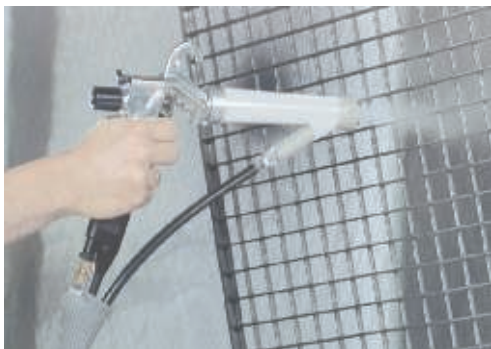
Figure 4 —Electrostatic spraying is well suited for metallic wire goods.
