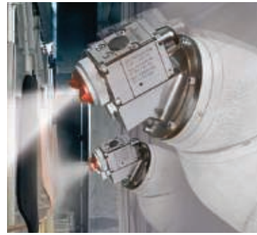
Figure 8— An HVLP gun provides excellent atomization and improved transfer efficiency.
