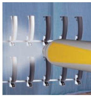
Figure 9— An electrostatic bell is used for exceptional film uniformity on automotive trim components.
