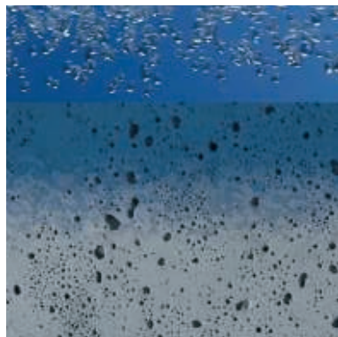
FIGURE 2—Color-based test for sealer penetration into concrete. 10
