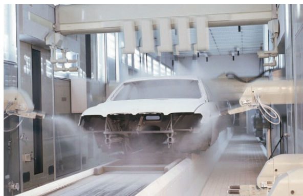
Figure 1 —Powder clearcoat automatically applied to a BMW 7-Series body. (Photo courtesy of BMW.)
