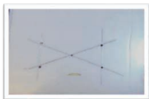
FIGURE 11A—RDPA-1 epoxy primer and polycarbamide topcoat applied after 60 min.
