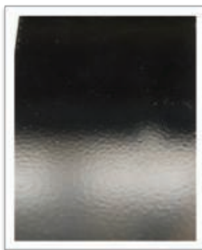
FIGURE 9A —Topcoat applied over phenalkamine epoxy primer.
