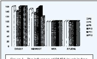
Figure 1—The influence of DMPA levels in free radical UV curable coatings. Direct and indirect impact (160 lb/in. = best); (solvent resistance: 100 double rubs = best).
