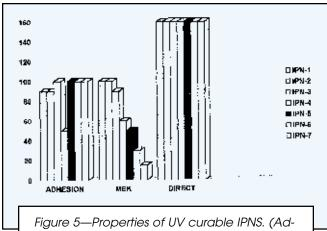
Figure 5—Properties of UV curable IPNS. (Adhesion: 10 = best; MEK resistance: 100 double rubs = best; direct impact: 160 lb/in = best).
