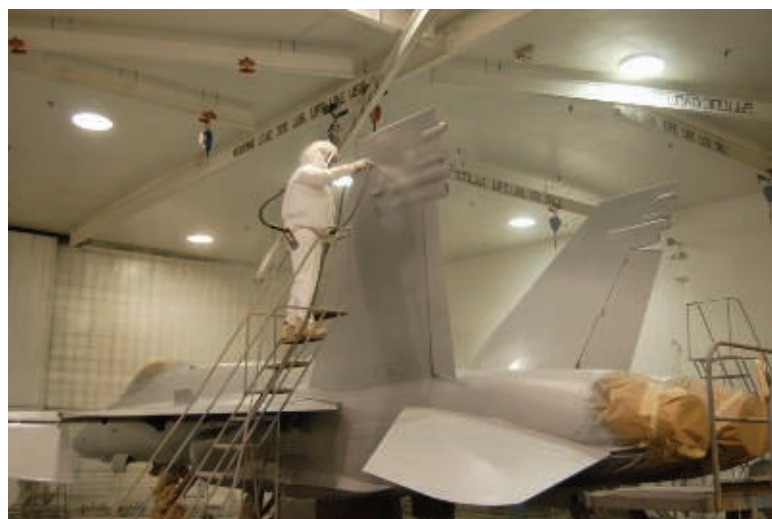
FIGURE 2— Spray application of a polyurethane topcoat on an F/A-18 aircraft.
