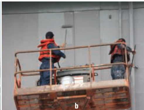
FIGURE 1— a: “Pinking” of an LSA haze gray silicone alkyd on the topside of a Navy surface ship; and b: sailors roll-applying fresh silicone alkyd over aged silicone alkyd.
