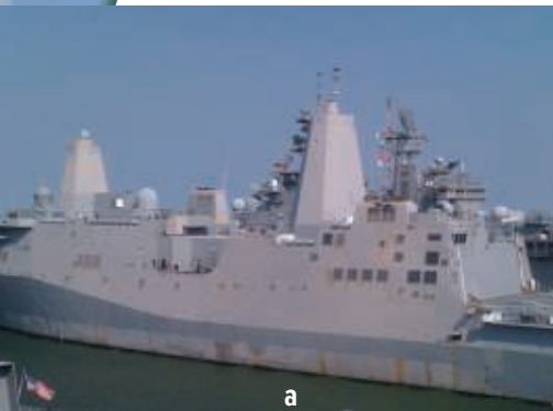
FIGURE 1— a: “Pinking” of an LSA haze gray silicone alkyd on the topside of a Navy surface ship; and b: sailors roll-applying fresh silicone alkyd over aged silicone alkyd.
