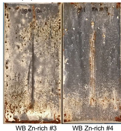
FIGURE 8 —Panel images after 2400-h salt spray exposure (surface rusts were removed via scratch pad).
