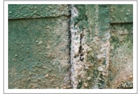
FIGURE 6—Coatings on southern yellow pine boards showing both poor (red box) and excellent grain crack resistance.
