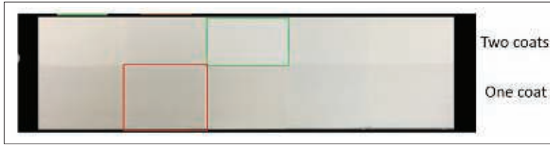
FIGURE 4—Tannin migration from Redwood to coatings. Superior performing polymers (green box) block tannin migration, as compared to one coat of an inferior paint (red box) where the brown color of the tannin migrates through.
