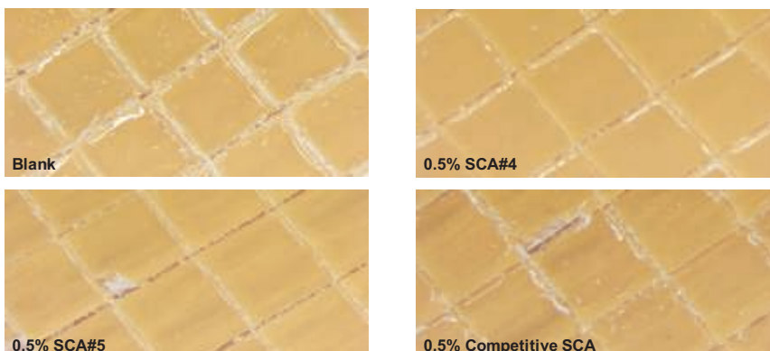
FIGURE 9—Comparison of cross-cut areas of panels that have been coated twice with pigmented waterborne acrylic wood coatings containing 0.5 wt% surface control additives.
